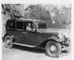
SIXTEEN/EIGHTEEN. 1933-34/1934 (prod: 5742/2630). 2-seater, tourer, various saloons. F/R, 2249cc/2511cc (S6 SV). Main improvements for '33 as for Heavy 12 and has silent 3rd 'box as fitted from January '32, though '34s have synchromesh. Mechanical pump feed replaces Autovac. Fourbearing 18HP alternative and optional 120ins wheelbase chassis from 1934. Connoisseurs of the bizarre shouldn't forget the Hayes automatic 'box option, of which about 50 sold, 1934-36.
