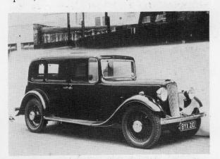
SIXTEEN/EIGHTEEN. 1935-36/1935-37 (prod: 12,731 all types). 5-seater saloon, 7-seater saloon. F/R, 2249cc/2511cc (S6 SV). New painted grilles, new projecting boots (full of spare wheel), synchromesh on 2nd, and both engines now with four mains only. Hayes transmission still available to '36, when down-draught carburettors standard. Only 18 offered in '37, main change being easy-clean instead of wire wheels.
