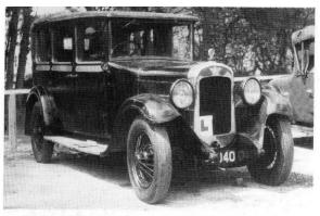
20 HP LONG. 1930-35 (prod: 3406 all 20 HP to 1934). Fabric saloon, limousine, landaulette. F/R, 3400cc (S6 SV). Big formal carriage on 136ins wheelbase, introduced 1927. Chromium plate and coil ignition 1930, rear tanks and ribbon radiator shells '31, further restyle '33, synchromesh '34, though Autovacs on all this series. No saloons after early '31, but Ranelagh limousine/landaulette carried over into '35 alongside later types. Artillery wheels available as well as wire.
