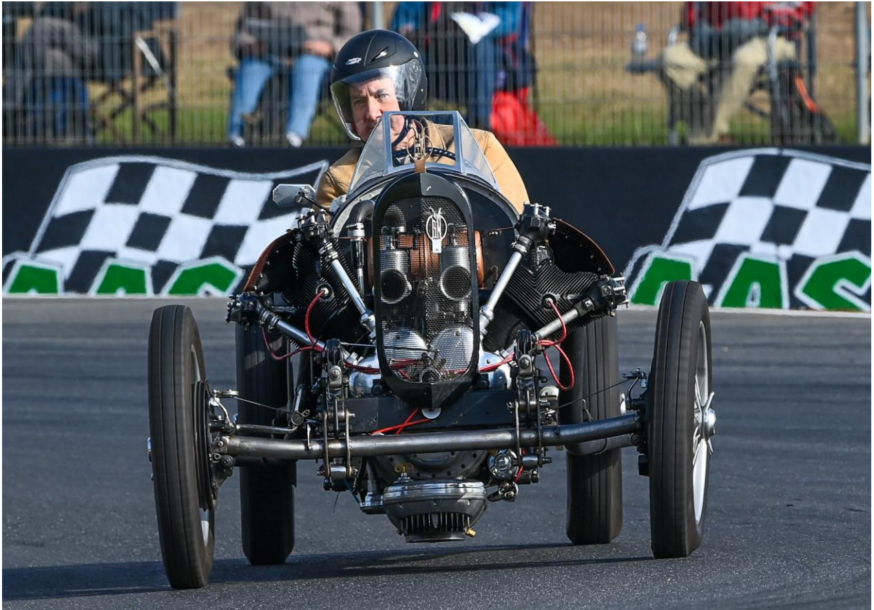
V Twin Built using Aircraft Cylinders.
